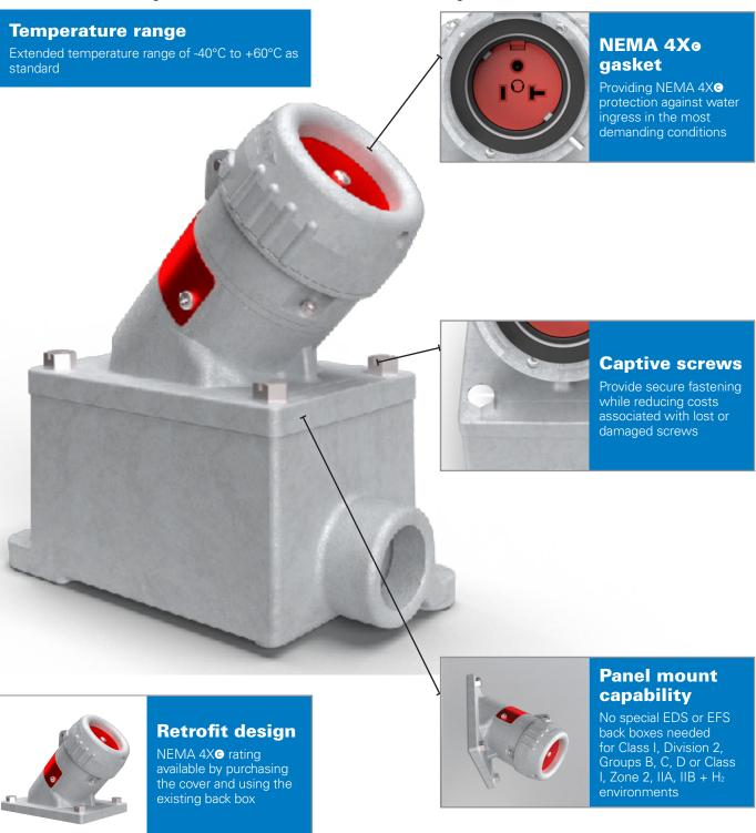
If existing back box is iron and is used with new X series cover, it is NEMA 4 rated. To achieve NEMA 4X rating, the back box and cover must be aluminum. For any questions, please contact your local sales rep or customer service.
