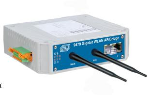
The 9479-ET-CSL is an Intrinsically Safe (IS) WLAN AP/Bridge Module suitable for Zone 1 / Zone 21 mounting, (Zone 0 / Zone 20 with a suitable Ex ia Power Supply).
