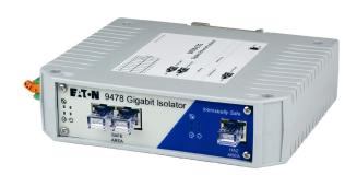
10/100/1000Mb\* IS Ethernet twisted pair (Cat5e/6) RJ45 connection (100metres length max.) provide total galvanic isolation (Um=253Vac) from safe to hazardous areas.
